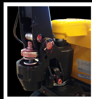
GREASE POINTS FOR EASE OF MAINTENANCE
