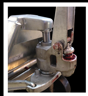
GREASE POINTS FOR EASE OF MAINTENANCE
