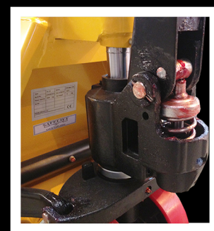
GREASE POINTS FOR EASE OF MAINTENANCE
